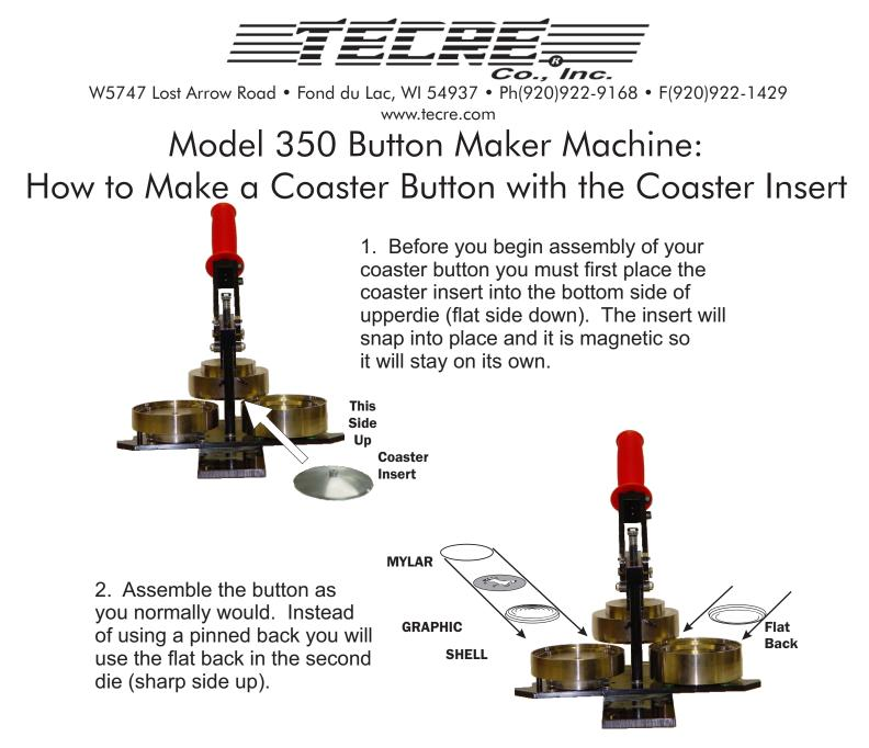
To remove the coaster insert, place the rod that came with the insert into the hole on top of the upper die. Press down and the insert will drop out of the upper die of the button maker.
