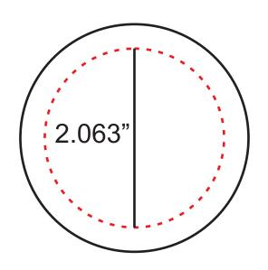
The second measurement is the live graphic area. This is the area that you will see on the face of the button. For a 2-1/4" the live graphic area is 2.063", as shown by the dashed line.
